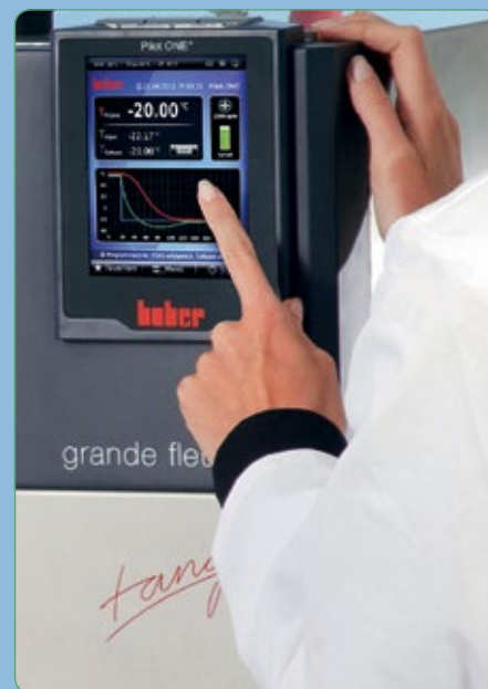
Fig. 3: Simple touch-screen operation of Pilot ONE models: memorable icons and a customizable Favourites menu make the operation intuitive and self-explanatory.
