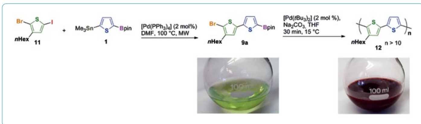
Scheme 2: Preparation of monomer 9a by nucleophile- and electrophile selective Stille cross-coupling reaction and subsequent polymerisation by Suzuki reaction.
