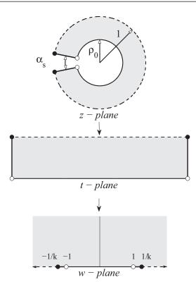
FIG. 8. The superconducting loop with a Josephson junction at the left. Schematically shown is the composition of conformal mapping transformations that convert the open annulus into the upper half-plane. Just for visual purposes, the width of the junction is oversized in the picture.
